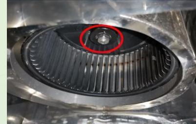
4 Adjust the motor position with gasket until the noise disappears /
